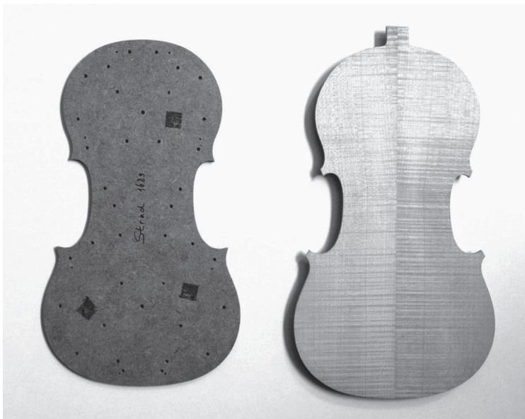
**Figure 1** Template (left) and backplate (right) of base model after Antonio Stradivari 1689.
